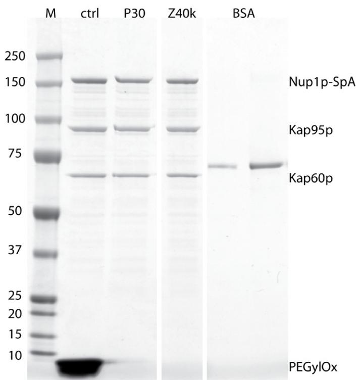
**Figure 1 – PEGyIOx depletion by spin column gel filtration with simultaneous buffer exchange:**
